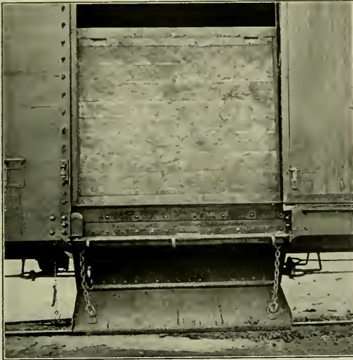
Exterior of Canadian Pacific Box Car with Hopper Open and Grain Door in Place.
